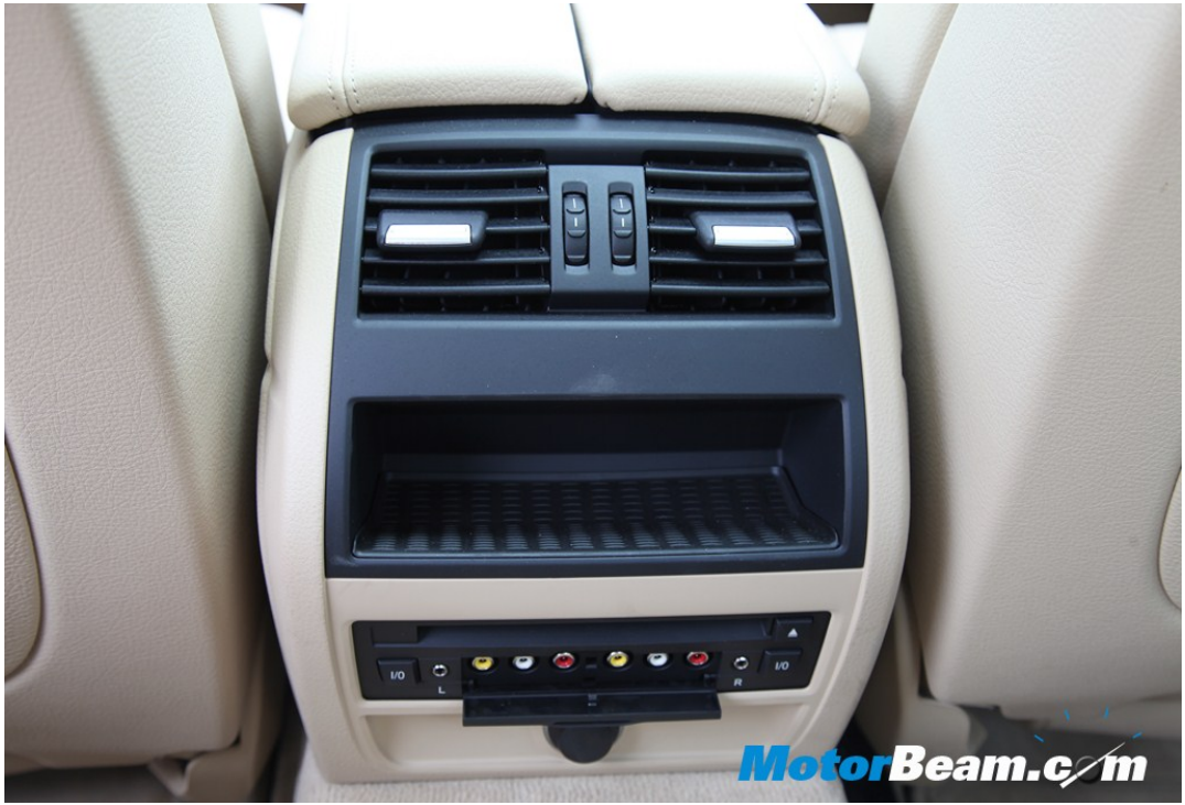
A DVD player is located in the central , console. Passengers can attach individual earphones and can enjoy music, videos etc from the iDrive or from their portable players through the RCA port.
