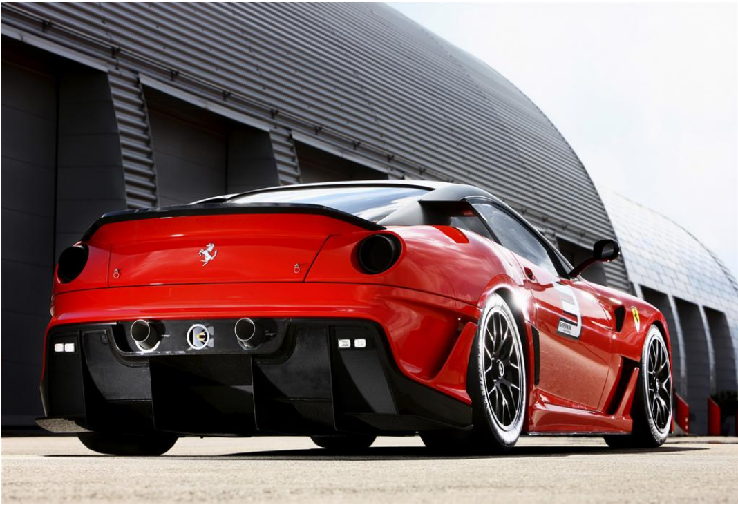
The Ferrari 599XX comes with slick tyres (29/67 R19 Front and 31/71 R19 Rear) specifically developed to
