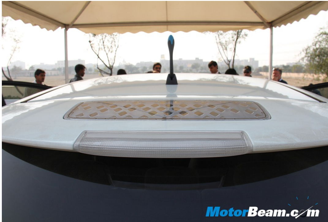
Solar Panel is optional. Notice the aerodynamically shaped antenna.
