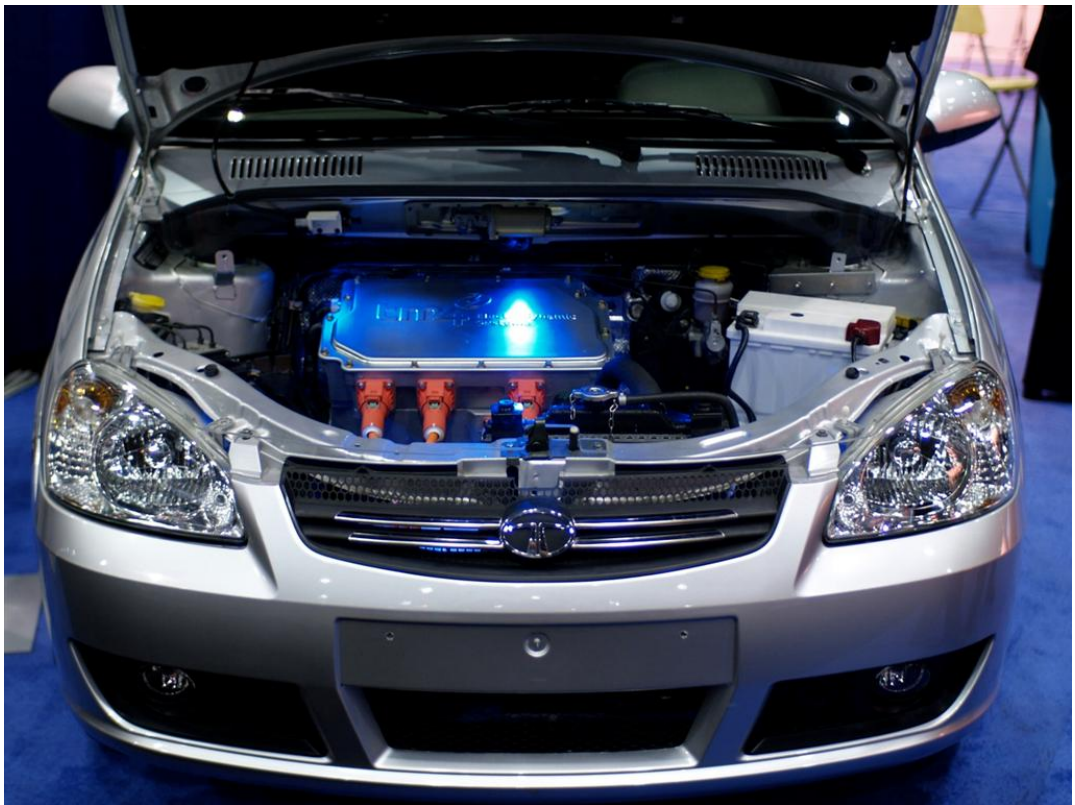
Tata's EV employs high capacity lithium ion batteries featuring what the brand calls super polymer cells. With these advanced power supplies, the small four-passenger car can travel 200 km (124 miles) on a single eight hour charge and can hit 60mph in a claimed less than 10 sec. After launching the Indica EV in Norway, Tata
