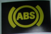
With the Anti-Lock Braking System (ABS), the car remains steerable even during sudden braking manoeuvres, and comes to a standstill as quickly as possible.
